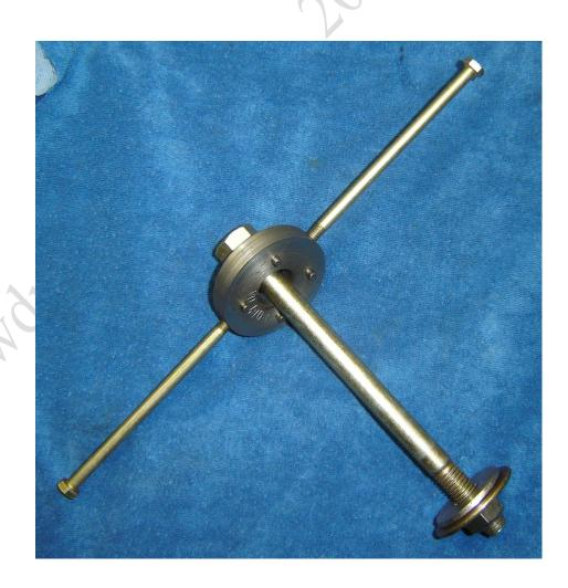
Drawing not to scale, dimensions Do and t are indicative. Picture shows final tool using long 6mm bolts as handles and a central 12 mm dia bolt which goes through the axle hole to clamp up the tool to the holes in the nut. Most of those holes are nackered and by clamping you can prevent initial slippage. When loosened, central bolt needs to be loosened also!
