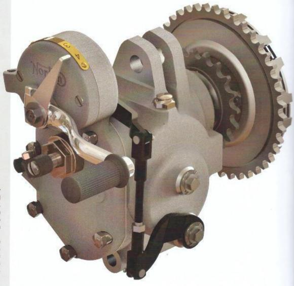
This gearbox is a Sturmey Archer by design, but is copied, improved and built by Burman for Norton. The four speed constant mesh close ratio gearbox has the two shafts positioned above each other.
