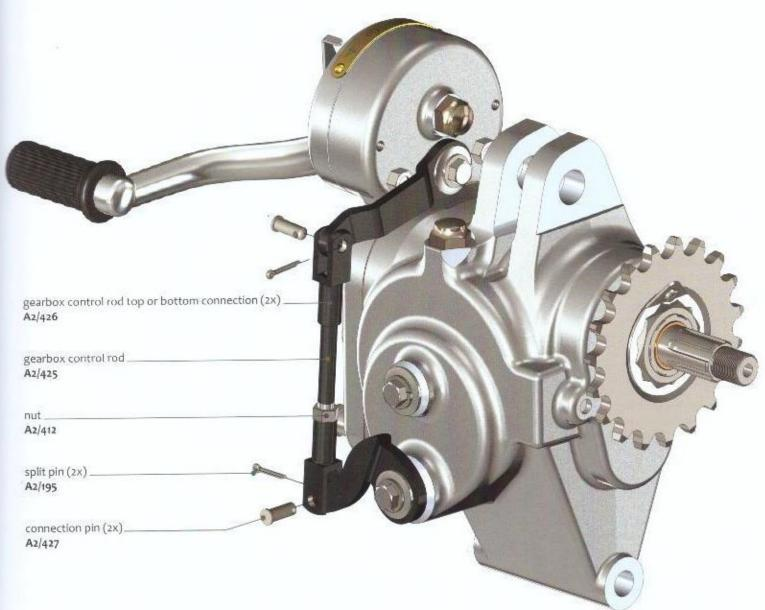
Before proceeding with the assembly steps that will take us to the clutch, it is good to have a closer look at what we have assembled so far, and see how the entire gearbox works. We start by looking at the positive foot change mechanism and make a random gear shift, in this case a shift upwards from 2<sup>nd</sup> to 3<sup>nd</sup> gear.
