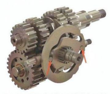
Mesh the striker fork dowels with the curved slots in the cam plate.
