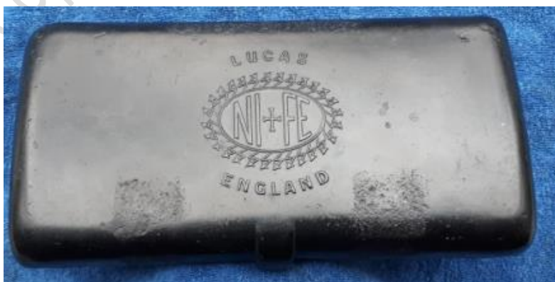
Top view showing the combined Lucas/Nife logo and wear marks from the battery carrier straps
