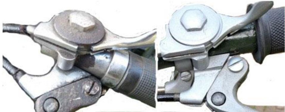
Early (left) and later (right) configuration of combination lever bodies
