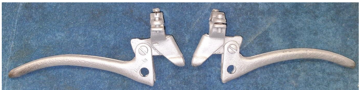
Folded assemblies part numbers LV7/BC/xx-xxx, for 7/8” handlebars
