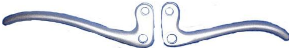
Front brake lever on the left (app. length 14,7 cm.) and clutch lever on the right (app. length 12 cm.).
