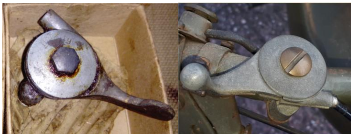
Air control pn 4102 versus Universal model air control LV7/BC/12-161
