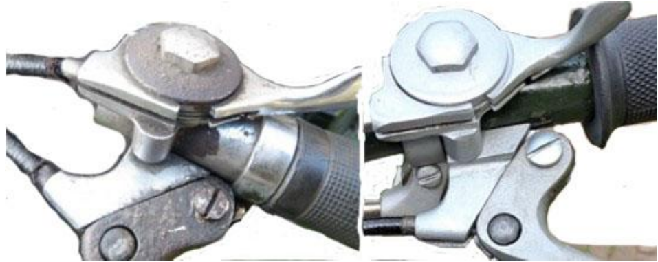
Early (left) and later (right) configuration of combination lever bodies
