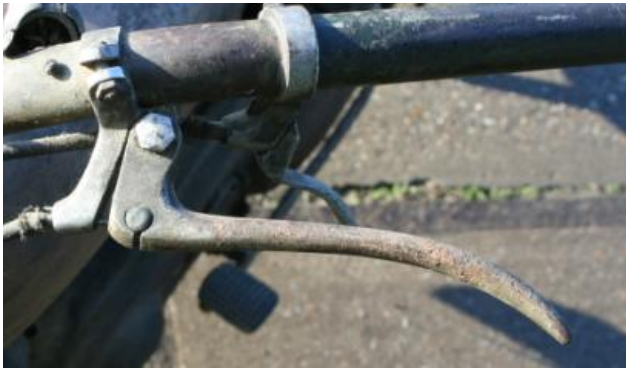
Solid body and clip, pn 3979 and multipurpose front brake and clutch lever pn 3980.
