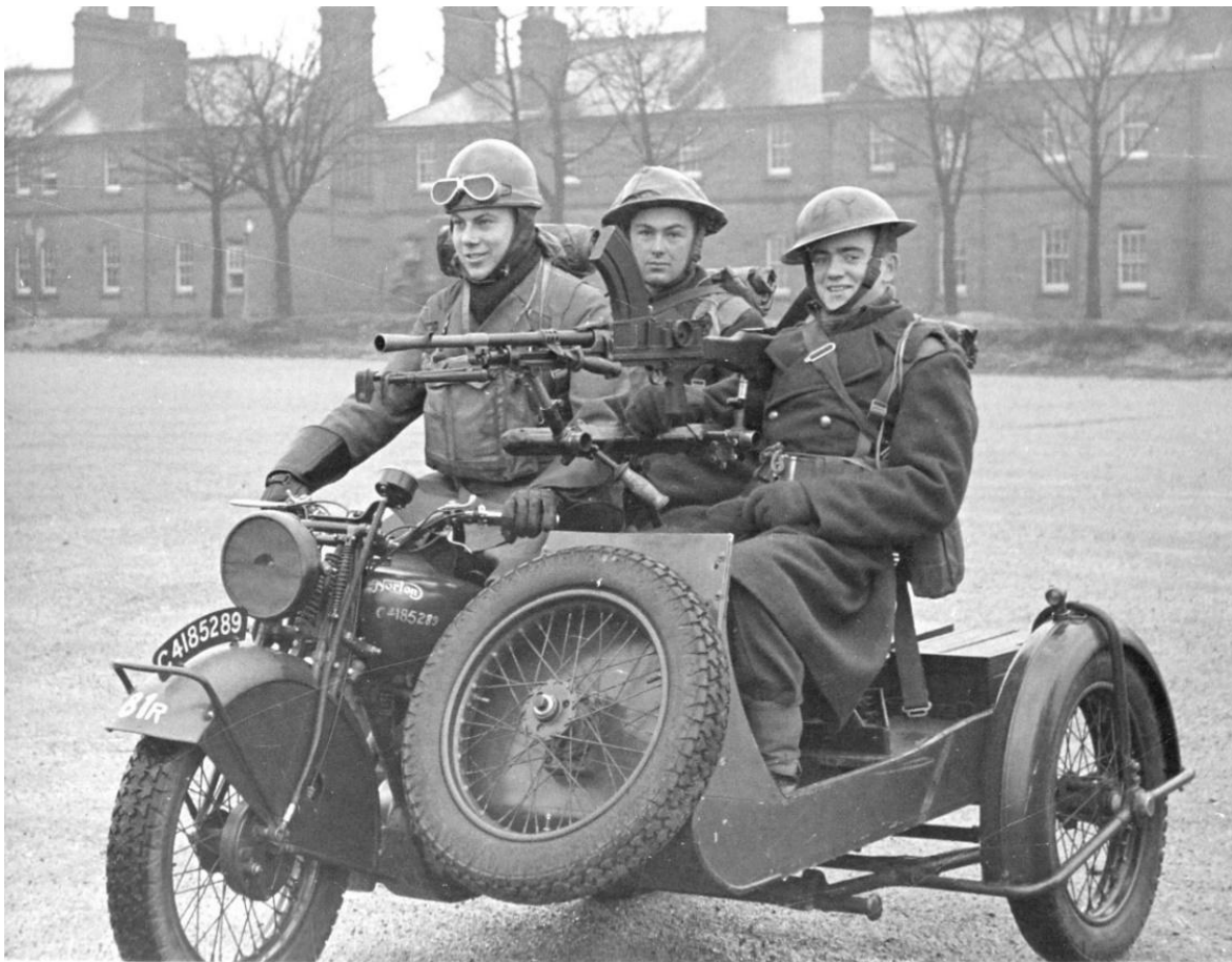
Contract V3849, C4185289, S1782 with Motley mount and smaller ammunition boxes at rear, spare wheel at front
