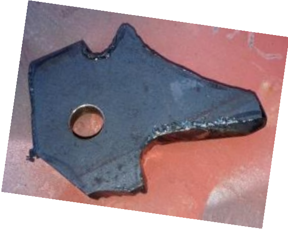
The first cut..... Using 1/4" flat steel, now for some filing!
