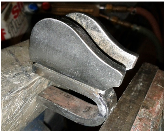
Using heat these two pieces were bent into shape 'tack' welded into place, filled with braze and filed down. The holes will come later.
